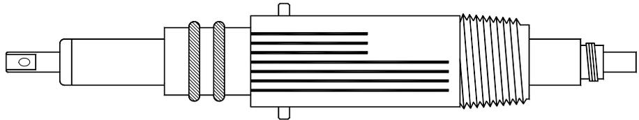
**Description:** The Tuff-Fet™ sensor is a solid state, ion sensitive field-effect transistor or ISFET. This technology does not require a glass membrane, making it perfect for Food-Grade Applications.
